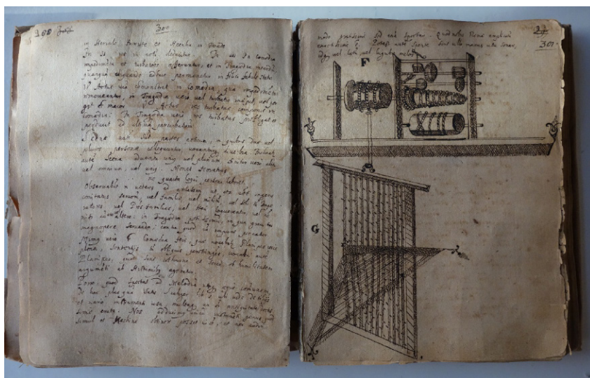
Figure 2. Design of a theatrical sound effects machine. A drawing from Maciej Kazimierz Sarbiewski's student lecture notes on poetics, 17th c. MNK Princes Czartoryski Library Ms. 1858.
