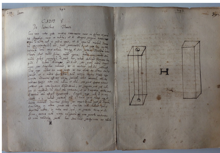
Figure 3. Design for rotating columns enabling sudden scene changes. A drawing from Maciej Kazimierz Sarbiewski's student lecture notes on poetics, 17th c. MNK Princes Czartoryski Library Ms. 1858.
